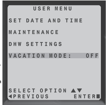
USER MENU screen — Scroll down to highlight VACATION MODE. Press ENTER key to set VACATION mode ON or OFF.
